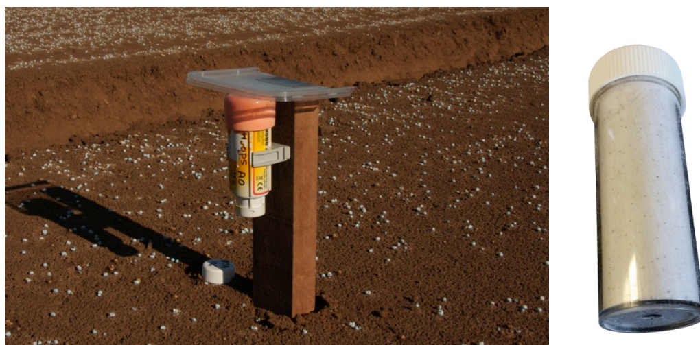
Figure 1 - Installation of temperature loggers: A Hobo UX100 was used to monitor air temperature and RH, while an i-button buried inside a small tube monitored soil temperature (only lid visible at left, i-button at base of tube at right).
