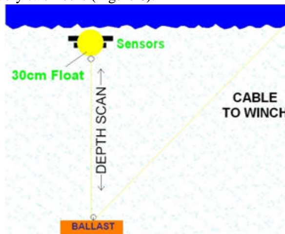
Figure 6. Datasonde depth scanning mechanism.
