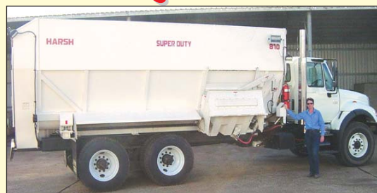
Harsh four auger mixers, truck and trailing
